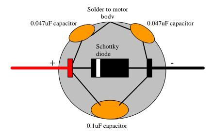
The above diagram shows a correctly suppressed motor. The capacitor values are not particularly critical but should be between .01uF and .1uF (microfarad). The voltage rating of each capacitor should be at least 5 times your cell pack voltage. The Schottky diode should have PIV rating of at least twice your cell pack voltage and have a maximum current rating (If) of at least 3 Amps. The diode must be omitted if the motor is connected to a reversing speed controller.
